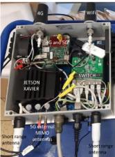
The Road Side Unit (fog node) integrates an Nvidia Jetson Xavier kit, that uses its GPU to timely detect a hazardous situation on the road, the communication modules and antennas, the power supply and all required connections. Finally, a camera along with a LiDAR unit are used to enhance the detection's precision and measure accurately the hazard's distance.
